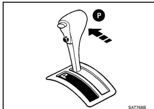
5. Does vehicle move when it is pushed forward or backward?
