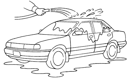
Water intrusion test
