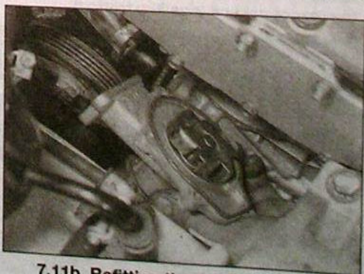
7.11b Refitting the coolant pump - 1.6 litre engine
