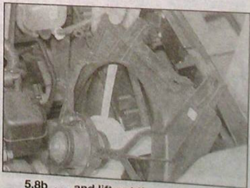
5.8b ... and lift out the cooling fan assembly
