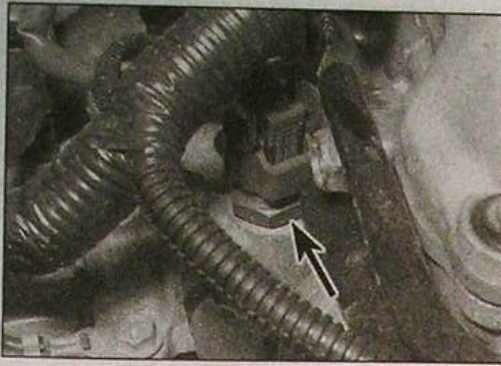
6.13 Engine temperature sensor (arrowed) - 1.6 litre fuel injection engine
