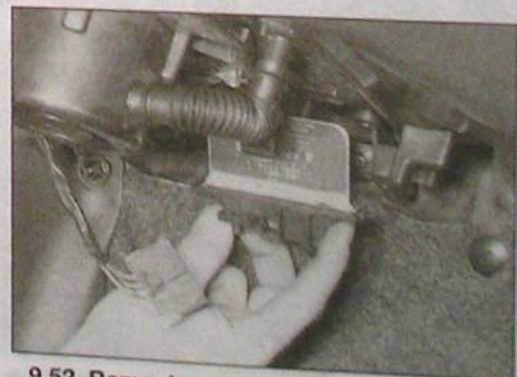
9.52 Removing the heater blower motor resistor
