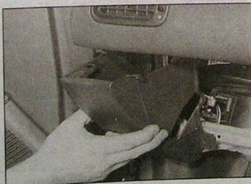
9.10 Removing the passenger's side lower facia panel
