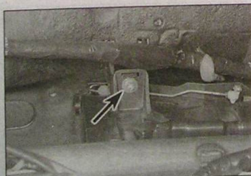
9.32b Heater assembly upper securing bolt (arrowed)
