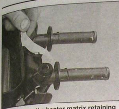
9.35 Remove the heater matrix retaining clip
