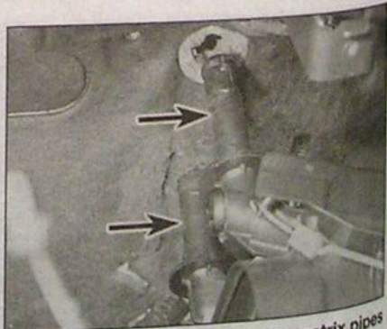
9.32d ... and pass the heater matrix pipes (arrowed) through the bulkhead
