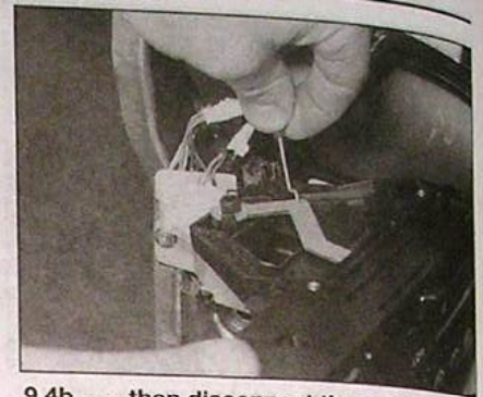
9.4b . . . then disconnect the control cable from the rear of the unit
