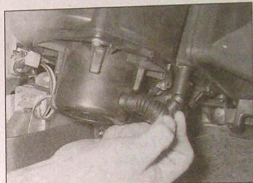
9.44 Disconnect the air hose from the motor casing ...
