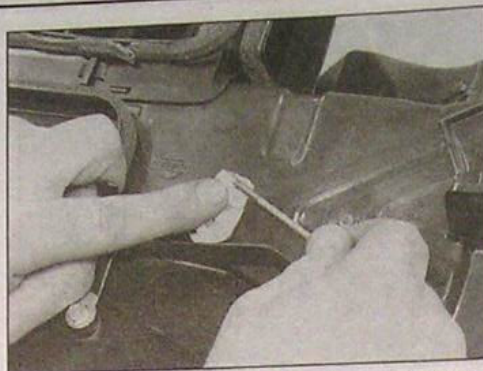
9.36 Disconnect the actuating rod from the lever on the heater assembly air flap
