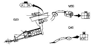
Fig. 20: Identifying Fuel Tank Sending Unit Connector Terminals Courtesy of Nissan Motor Co., U.S.A.
