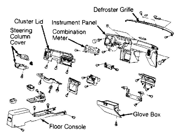
Fig. 24: Exploded View Of Instrument Panel (M30) Courtesy of Nissan Motor Co., U.S.A.
