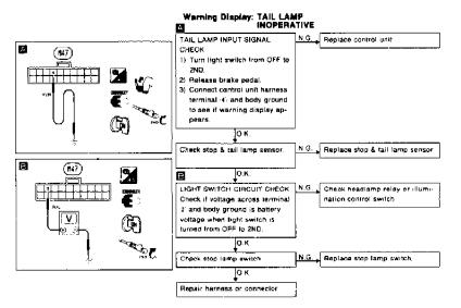
Fig. 11: Diagnosing Taillight Warning Displays (Q45) Courtesy of Nissan Motor Co., U.S.A.
