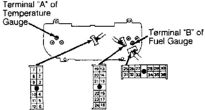
Fig. 19: Rear View Of Instrument Cluster (Q45) Courtesy of Nissan Motor Co., U.S.A.
