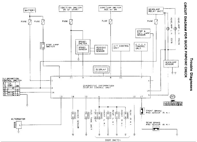
Fig. 2: Diagnostic Warning Light Wiring Schematic (Q45) Courtesy of Nissan Motor Co., U.S.A.
