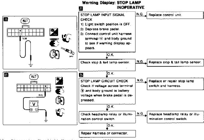
Fig. 10: Diagnosing Stoplight Warning Displays (Q45) Courtesy of Nissan Motor Co., U.S.A.
