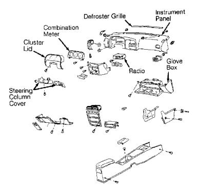
Fig. 23: Exploded View Of Instrument Panel (G20) Courtesy of Nissan Motor Co., U.S.A.
