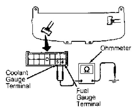
Fig. 17: Check Resistance Between Instr. Cluster Terminal & Ground (G20) Courtesy of Nissan Motor Co., U.S.A.
