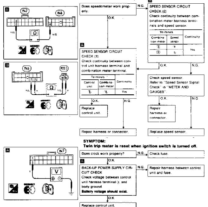
SYMPTOM: Twin tripmeter does not work. (Remains at "0" or some number and does not accumulate.)
