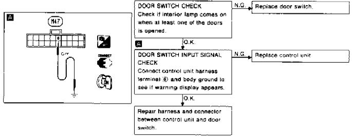
Fig. 6: Diagnosing Door Open Warning Displays (Q45) Courtesy of Nissan Motor Co., U.S.A.
