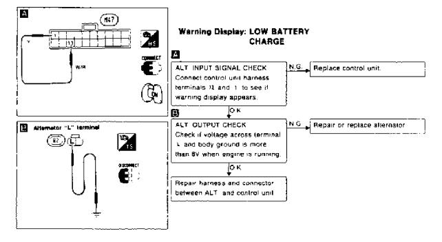
Fig. 13: Diagnosing Low Battery Charge Warning Displays (Q45) Courtesy of Nissan Motor Co., U.S.A.
