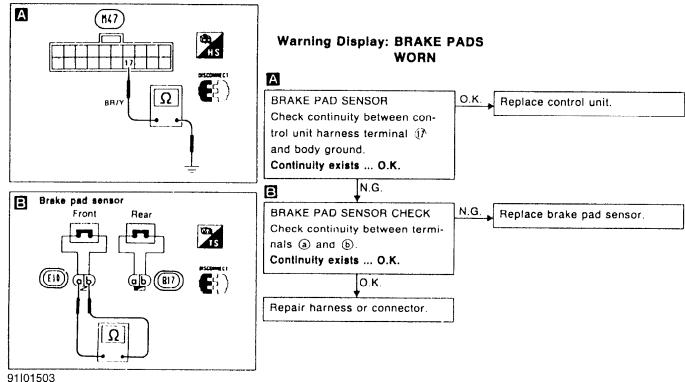
Fig. 14: Diagnosing Brake Pads Worn Warning Displays (Q45) Courtesy of Nissan Motor Co., U.S.A.
