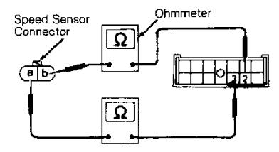
Fig. 22: Testing Speed Sensor Continuity (Q45 Shown; M30 Similar) Courtesy of Nissan Motor Co., U.S.A.
