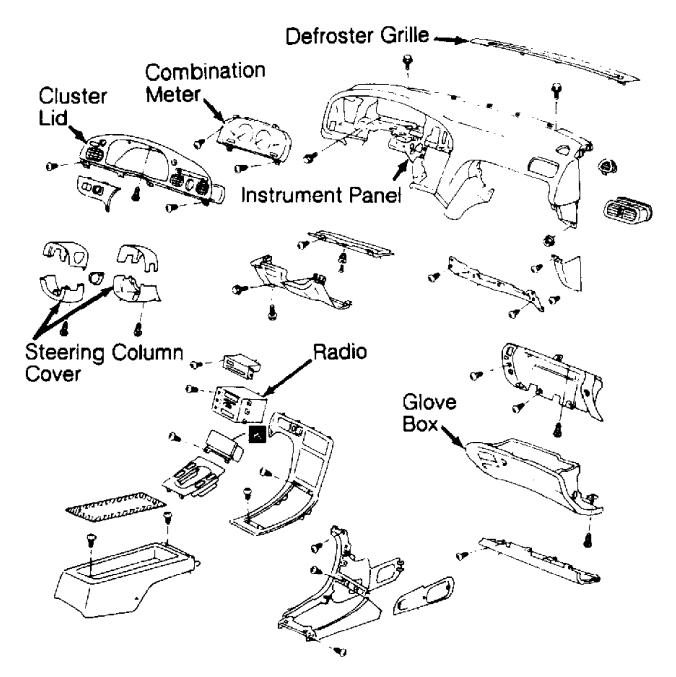
Fig. 25: Exploded View Of Instrument Panel (Q45) Courtesy of Nissan Motor Co., U.S.A.
