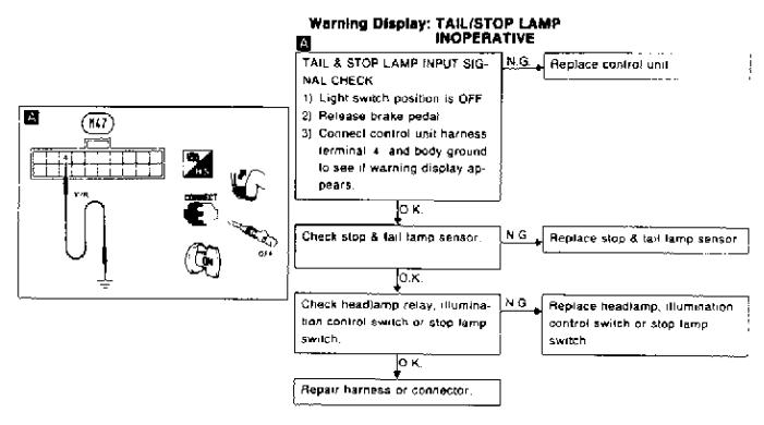
Fig. 12: Diagnosing Taillight/Stoplight Warning Displays (Q45) Courtesy of Nissan Motor Co., U.S.A.
