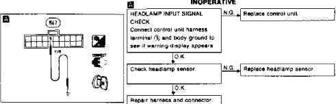
Fig. 9: Diagnosing Headlight Warning Displays (Q45) Courtesy of Nissan Motor Co., U.S.A.
