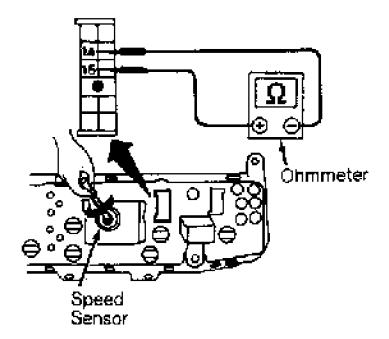
Fig. 21: Testing Speed Sensor Continuity (G20) Courtesy of Nissan Motor Co., U.S.A.
