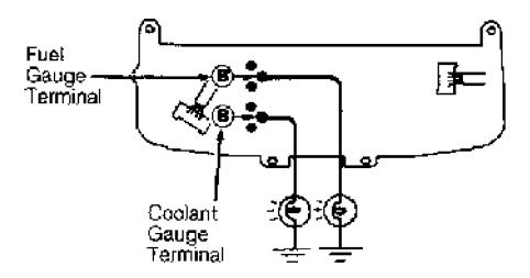
Fig. 16: Testing Fuel & Temperature Gauges (G20) Courtesy of Nissan Motor Co., U.S.A.
