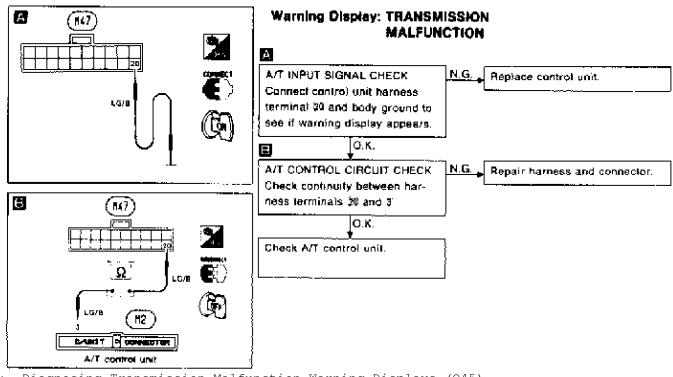
Fig. 5: Diagnosing Transmission Malfunction Warning Displays (Q45) Courtesy of Nissan Motor Co., U.S.A.
