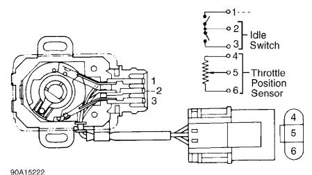
Fig. 7: Testing Throttle Position Sensor Courtesy of Nissan Motor Co., U.S.A.
