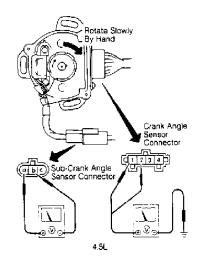
Fig. 6: Crankshaft Angle Sensor Terminal ID (Q45) Courtesy of Nissan Motor Co., U.S.A.
