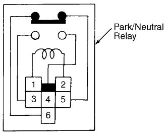
90C15224 Fig. 9: Park/Neutral Relay Terminal ID (Q45) Courtesy of Nissan Motor Co., U.S.A.
