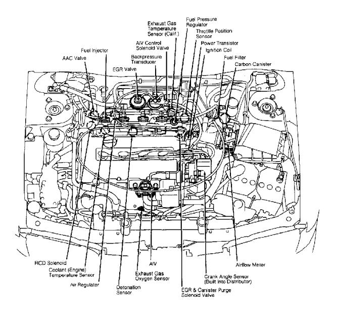
Fig. 17: Underhood Engine Performance Component Locations (G20) Courtesy of Nissan Motor Co., U.S.A.
