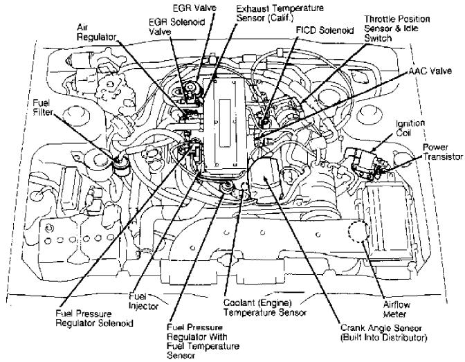
Fig. 18: Underhood Engine Performance Component Locations (M30) Courtesy of Nissan Motor Co., U.S.A.
