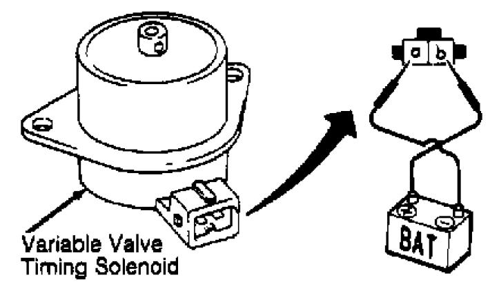
Fig. 16: Energizing Variable Valve Timing Solenoid Courtesy of Nissan Motor Co., U.S.A.
