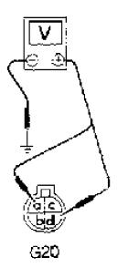
Fig. 4: Crankshaft Angle Sensor Terminal ID (G20) Courtesy of Nissan Motor Co., U.S.A.
