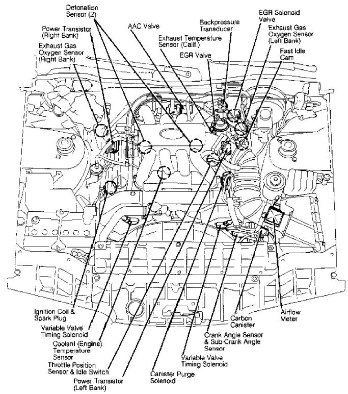
Fig. 19: Underhood Engine Performance Component Locations (Q45) Courtesy of Nissan Motor Co., U.S.A.
