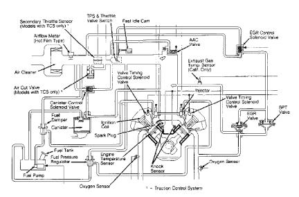
Fig. 3: Vacuum Diagram (Q45) Courtesy of Nissan Motor Co., U.S.A.
