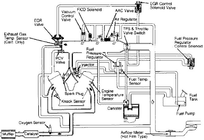
Fig. 2: Vacuum Diagram (M30) Courtesy of Nissan Motor Co., U.S.A.
