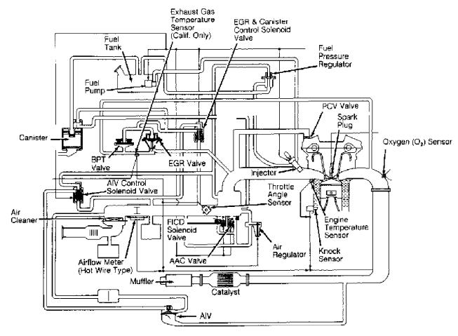
Fig. 1: Vacuum Diagram (G20) Courtesy of Nissan Motor Co., U.S.A.
