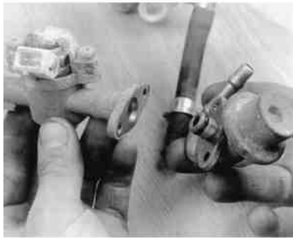
Fig. 2: Always replace the O-ring for the fuel pressure regulator
