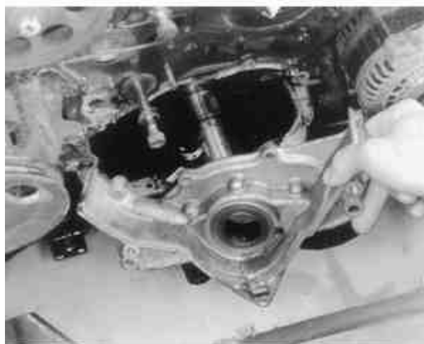
Fig. 7: Remove the oil pump pick-up tube assembly mounting bolts — 6-cylinder engines
