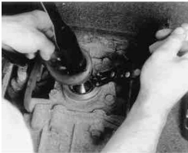
Fig. 5: Remove the shift lever from the transmission assembly
