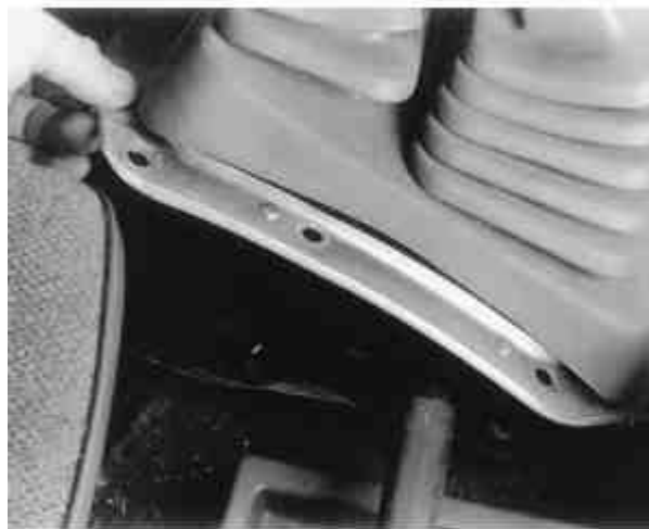
Fig. 3: The boot must be lifted for access to the shifter circlip
