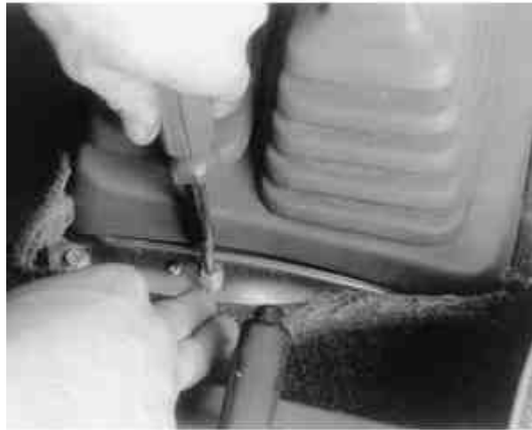
Fig. 2: After removing the screws, lift the retainer ring up
