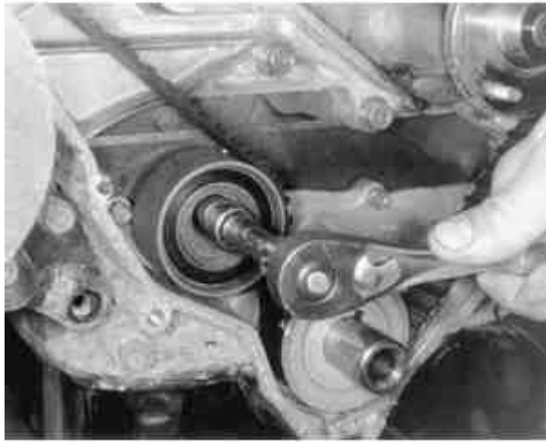
Fig. 16: Note the proper belt routing during removal
