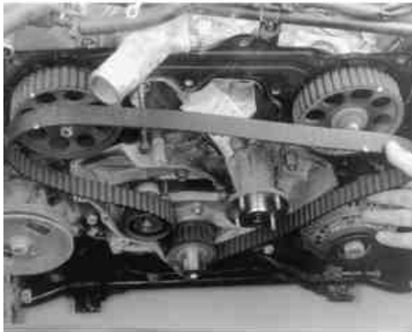
Fig. 17: Removing the water pump mounting bolts
