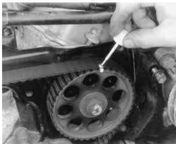
Fig. 15: Release the timing belt tensioner assembly
