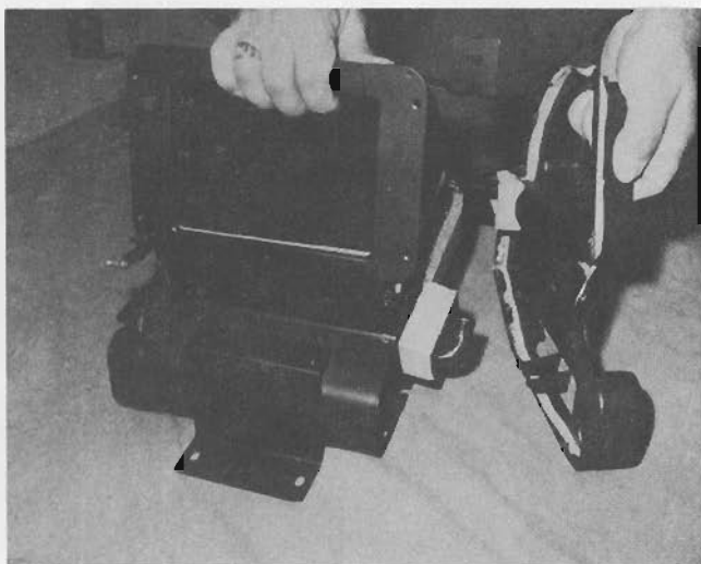
Figure III-12. Removing Heater End Plate
