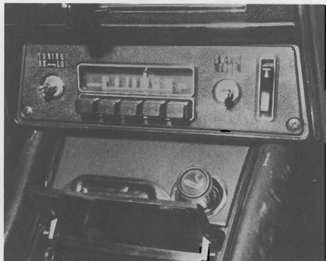
Figure V-2. Radio Tuner Mounting Screws
