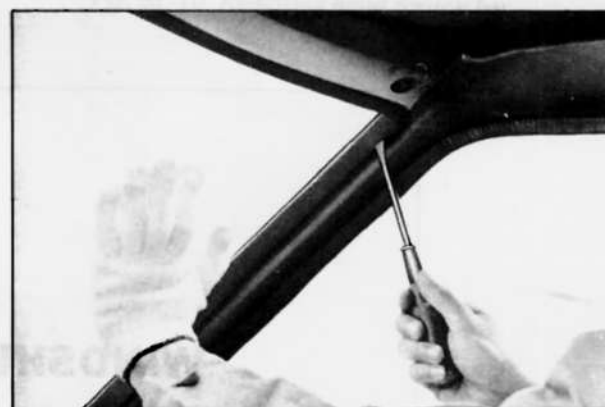
Fig. BF-14 Removing front windshield glass
