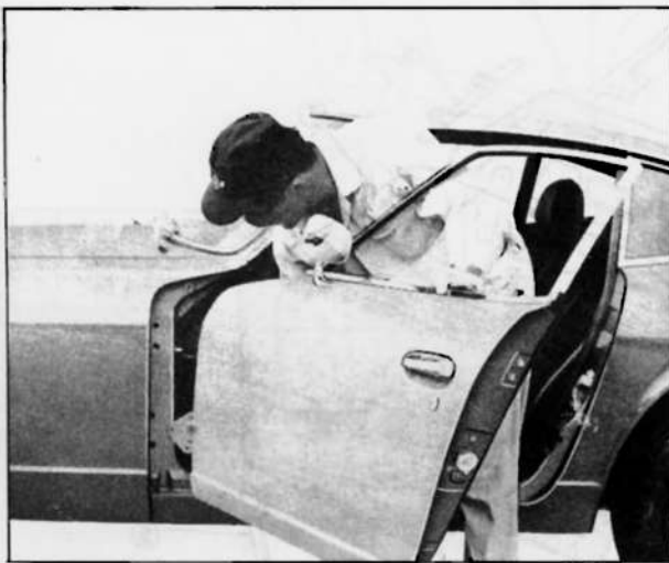
Fig. BF-19 Removing the door
