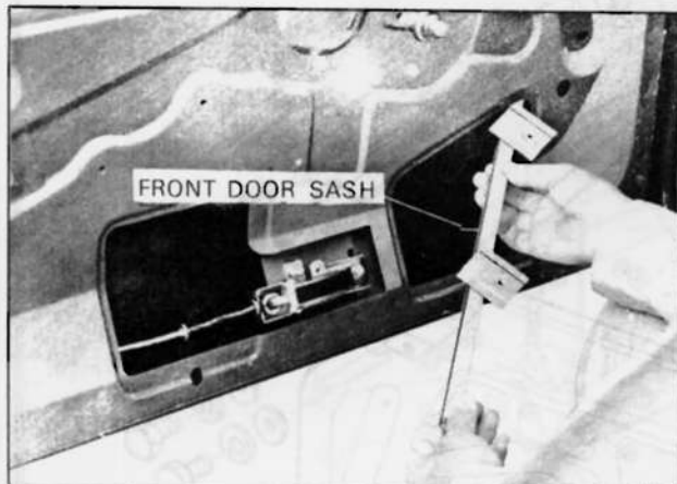
Fig. BF-29 Removing front door sash
