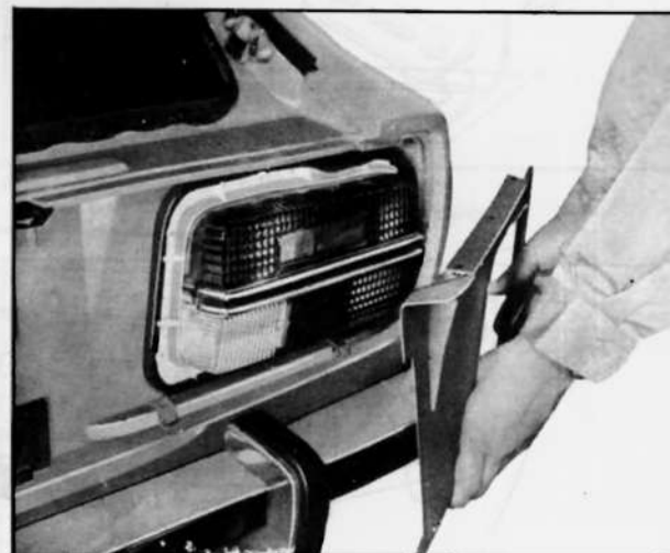
Fig. BF-47 Removing rear panel finisher
