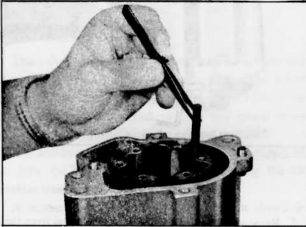
Fig. EC-13 Removing carbon shoe
