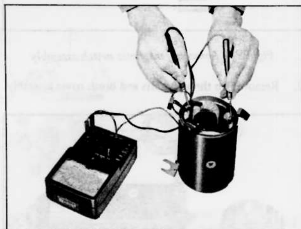
Fig. EE-12 Field coil test for continuity
