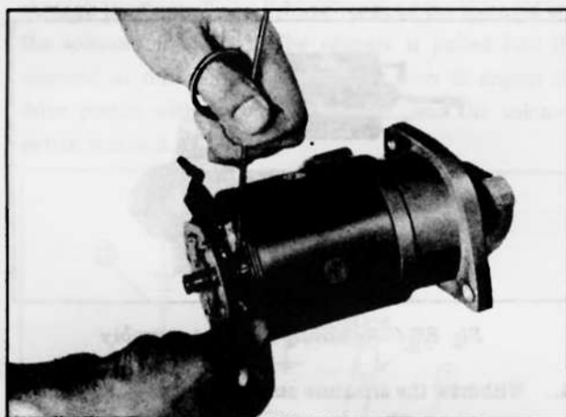
Fig. EE-9 Removing brush
