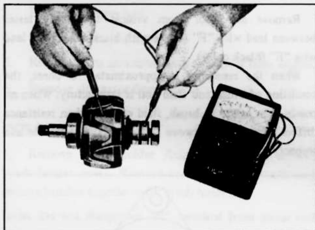
Fig. EE-41 Testing rotor coil for grounding
