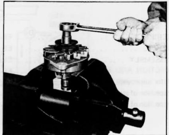
Fig. EE-33 Removing pulley and fan
