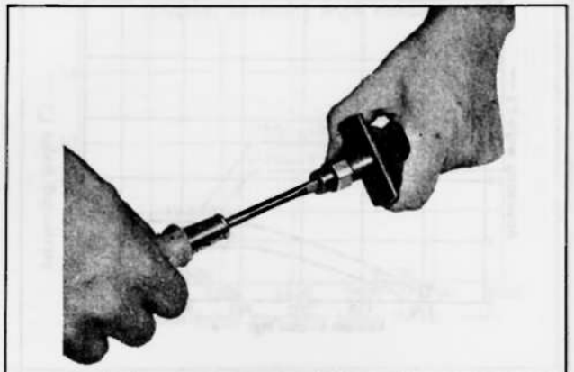
Fig. EE-76 Removing cam
