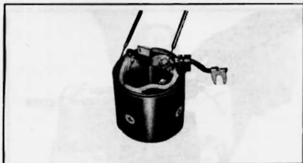
Fig. EE-13 Field coil test for grounding
