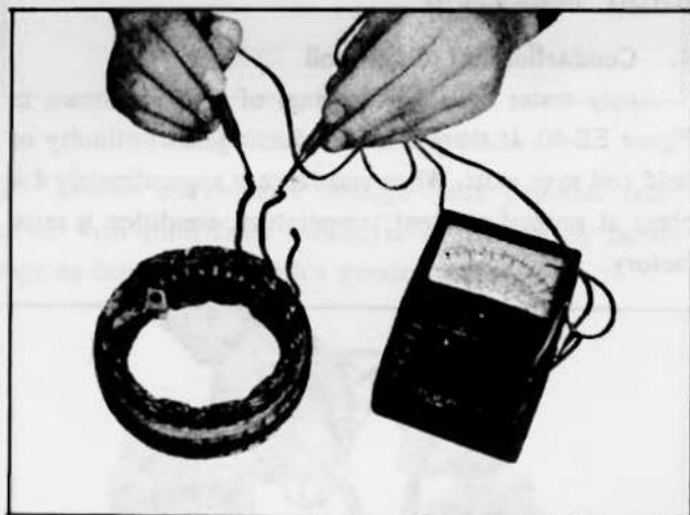
Fig. EE-42 Testing stator for conduction
