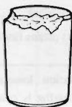
d) Cracked roller
