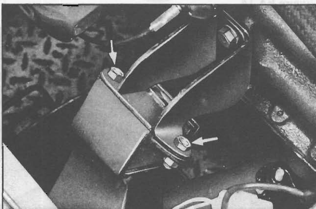
Fig. FA-7 Removing engine mounting bolts
