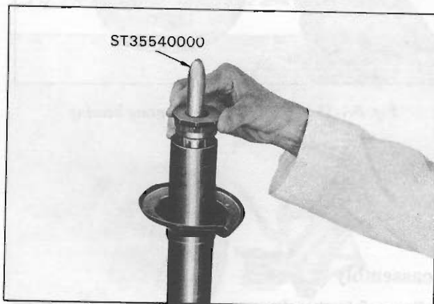
Fig. FA-35 Installing gland packing
