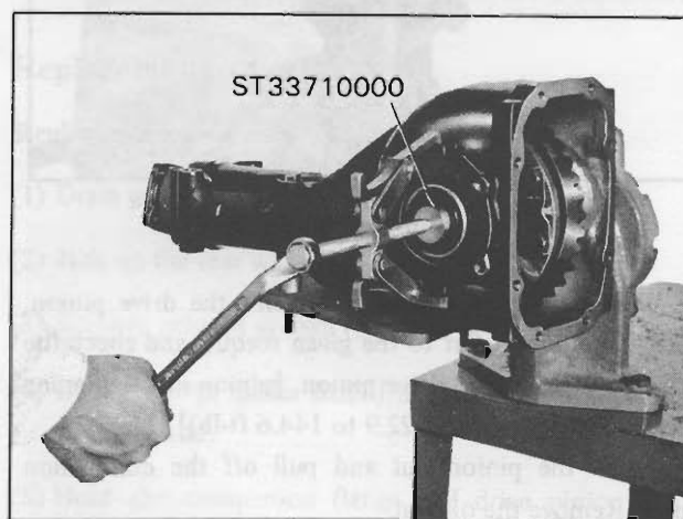
Fig. PD-5 Removing side retainer
