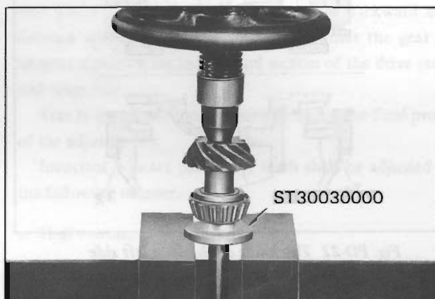
Fig. PD-20 Pressing rear bearing inner race
