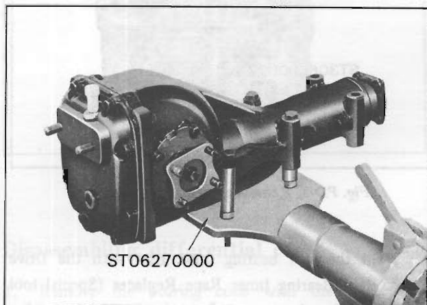
Fig. PD-3 Holding differential carrier
