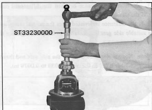
Fig. PD-17 Pressing side bearing cone
