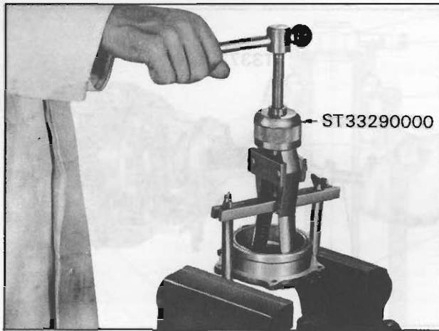
Fig. PD-6 Removing side bearing outer race
