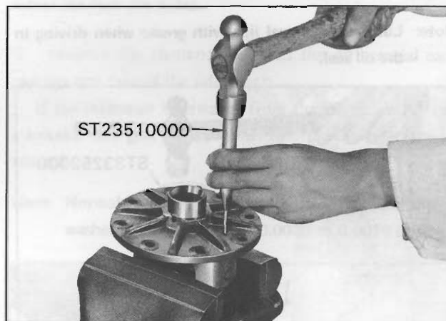
Fig. PD-12 Punching off lock pin
