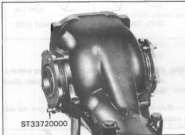
Fig. PD-25 Installation of side retainer
