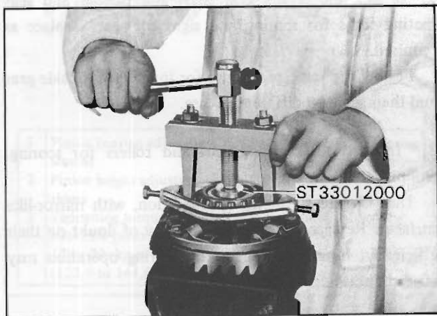
Fig. PD-11 Removing side bearing cone
