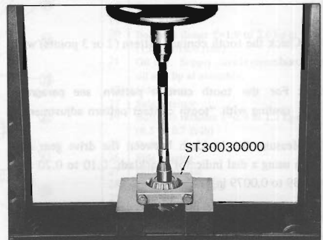
Fig. PD-9 Removing rear bearing inner race
