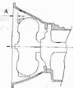
Fig. AT-50 Installing torque converter
