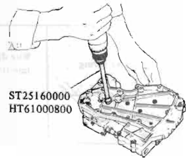
Fig. AT-108 Installing valve body
