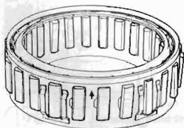
Fig. AT-71 One-way clutch
