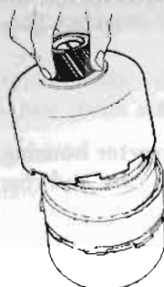
Fig. AT-73 Installing connecting shell
