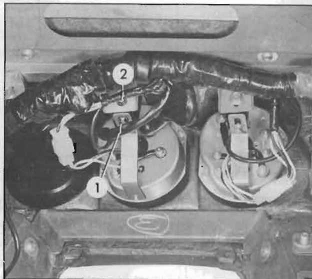
Fig. BE-22 Removing ammeter and fuel gauge
