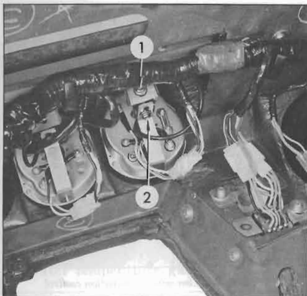
Fig. BE-20 Removing water temperature gauge and oil pressure gauge
