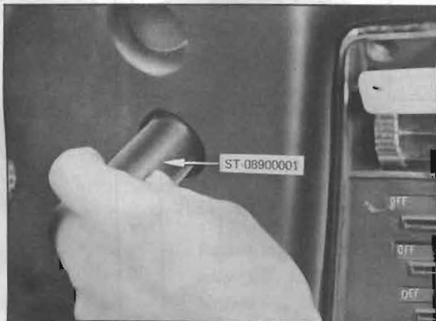
Fig. BE-31 Removing switch
