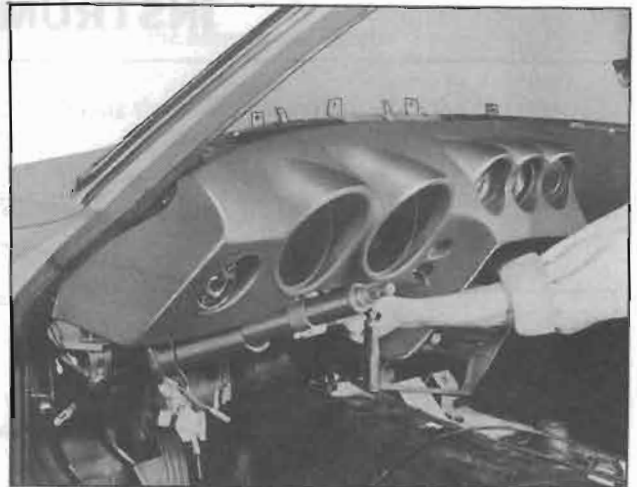
Fig. BF-53 Removing instrument
