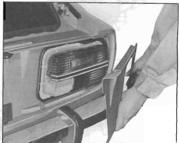
Fig. BF-50 Removing rear panel finisher
