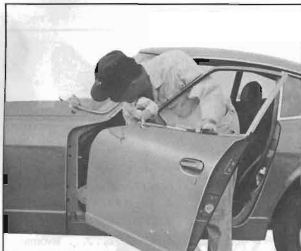
Fig. BF-22 Removing the door
