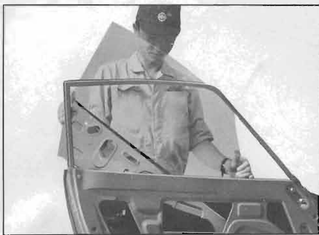
Fig. BF-33 Removing door glass
