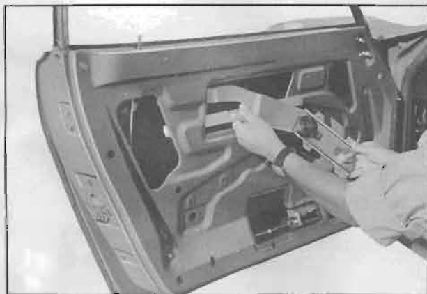
Fig. BF-34 Removing door window regulator
