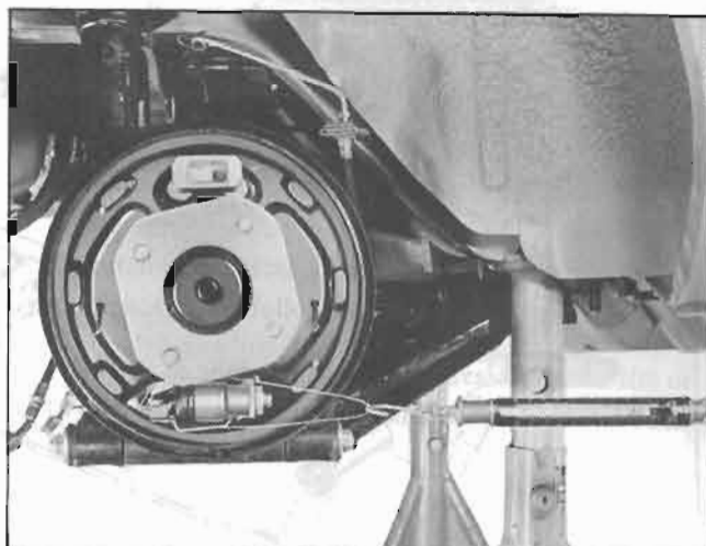
Fig. BR-32 Measuring sliding resistance
