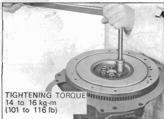
Fig. EM-80 Flywheel installation
