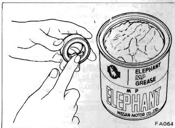
Fig. FA-33 Greasing strut mounting bearing
