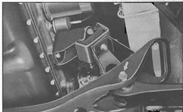
Fig. FA-44 Loosening transverse link mounting bolt
