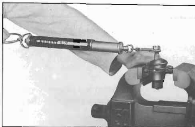
Fig. FA-47 Measuring ball joint shaking torque
