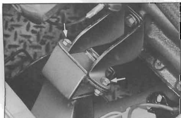
Fig. FA-7 Removing engine mounting bolts
