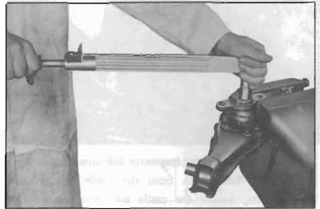
Fig. FA-48 Tightening knuckle arm castle nut
