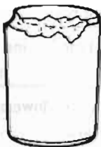
d) Cracked roller
