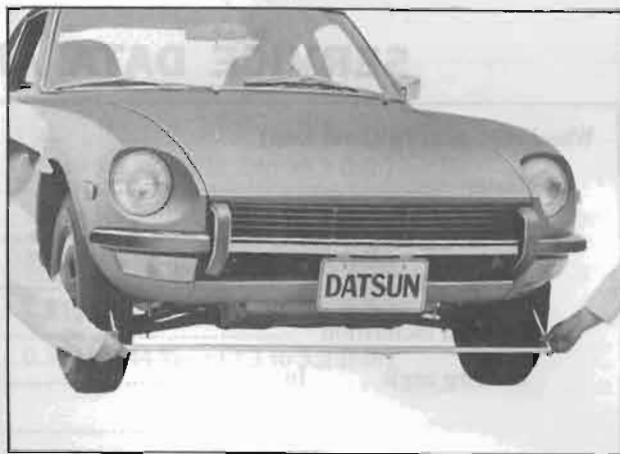
Fig. FA-50 Measuring toe-in
