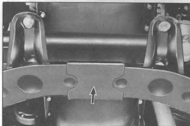
Fig. FA-8 Jack-up point of suspension cross member
