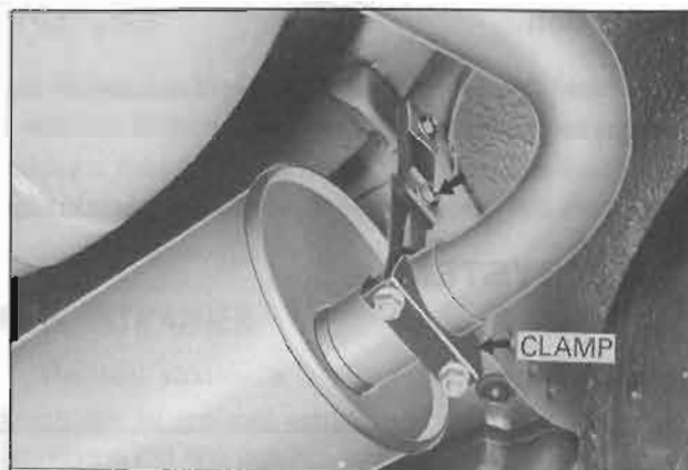
Fig. FE-6 Removing exhaust hanger strap (point "D")
