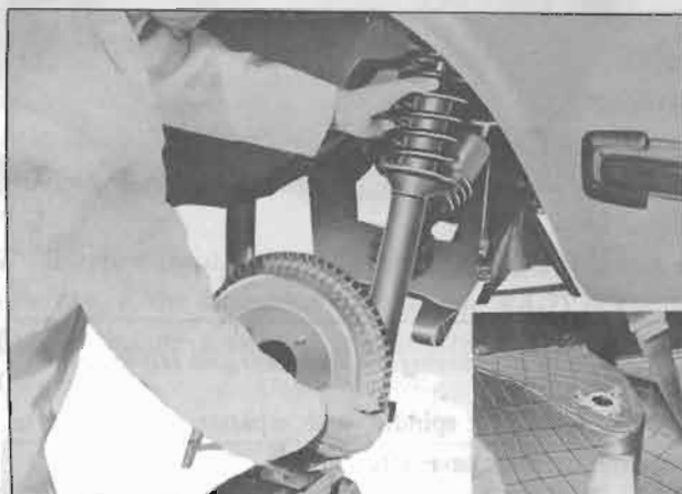
Fig. RA-14 Removing the strut assembly
