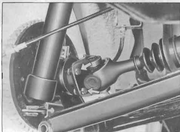
Fig. RA-13 Removing the drive shaft
