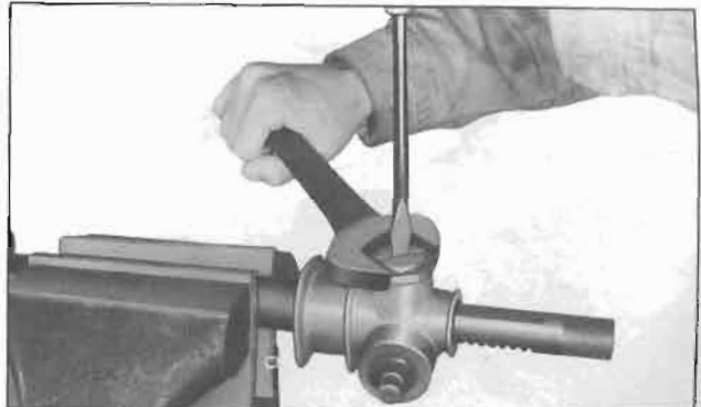
Fig. ST-33 Locking retainer lock nut
