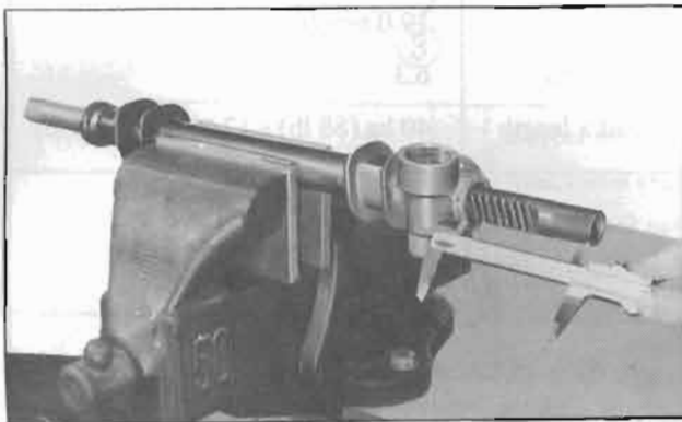
Fig. ST-26 Measuring protruding portion of rack
