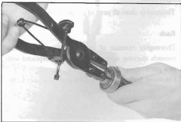
Fig. ST-22 Removing snap ring
