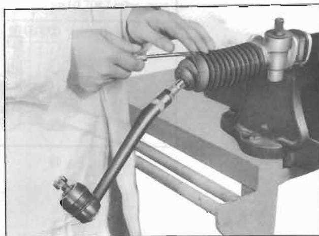
Fig. ST-16 Removing dust cover clamp
