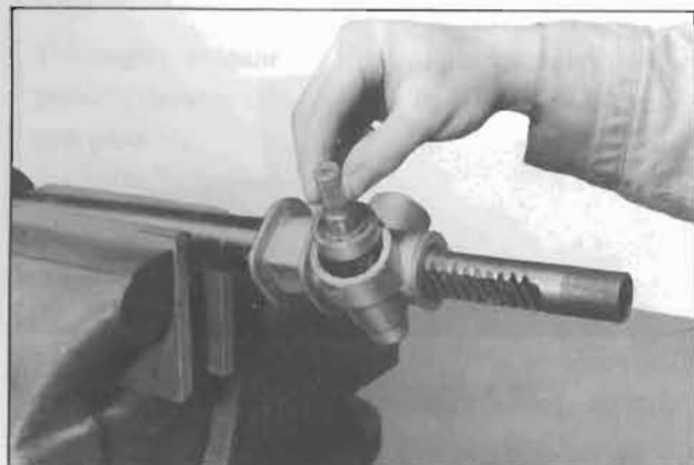
Fig. ST-27 Inserting pinion
