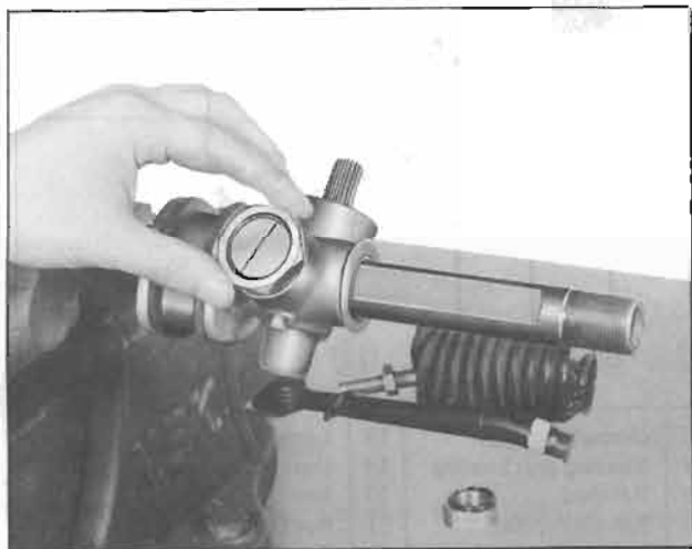
Fig. ST-18 Removing side rod outer socket
