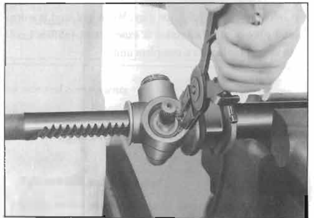
Fig. ST-29 Fitting snap ring
