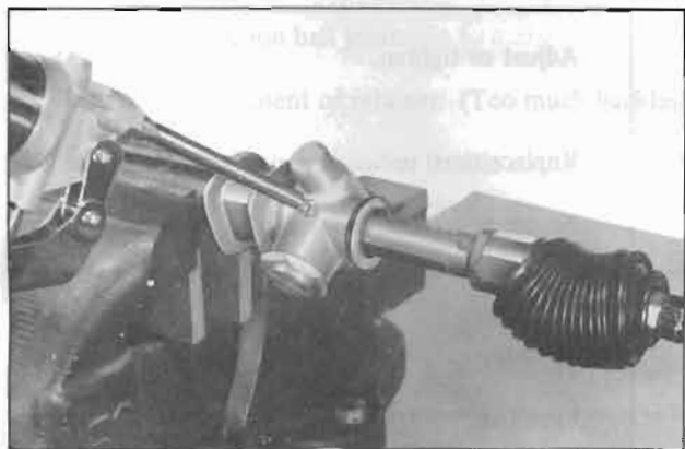
Fig. ST-40 Supplying the grease
