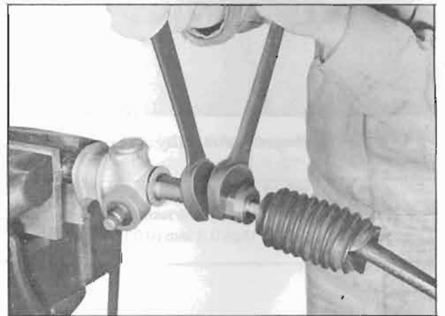
Fig. ST-38 Locking the stopper nut
