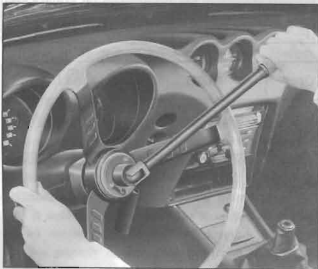
Fig. ST-3 Removing steering wheel
