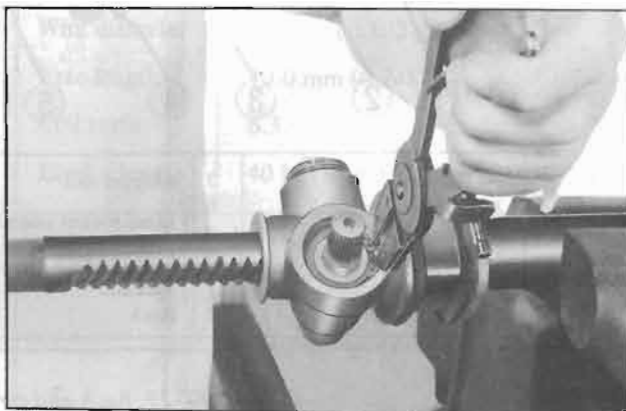
Fig. ST-21 Removing snap ring
