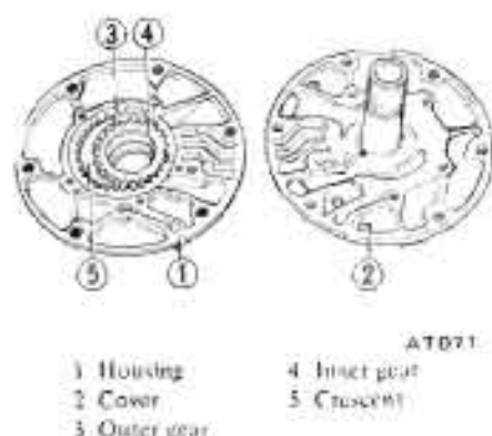
Fig. AT-3 Oil pump
