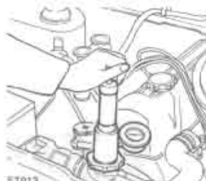
Fig. CO-11 Testing cooling system pressure
