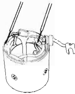
Fig. EE-17 Testing field coil for ground
