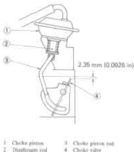
Fig. EF-54 Choke piston adjustment
