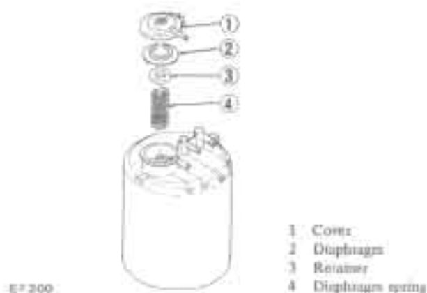
Fig. EF-66 Carbon canister purge control valve
