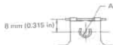
Fig. EF-46 Measuring "H" dimension at point A
