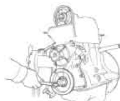
Fig. EM-101 Installing crankshaft pulley
