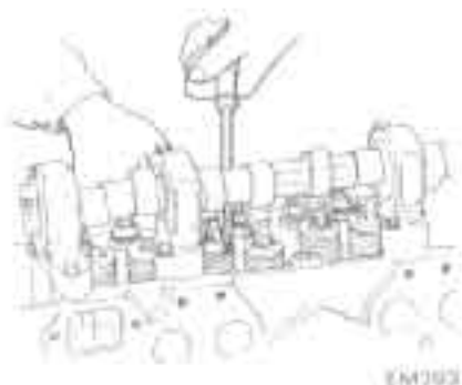
Fig. EM-26 Removing rocker arm
