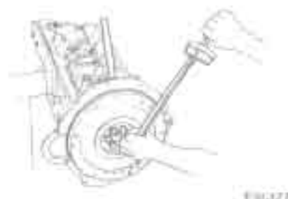
Fig. EM-91 Installing flywheel
