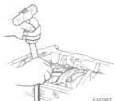
Fig. EM-60 Checking crankshaft end play
