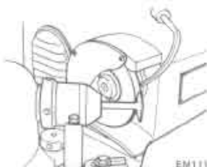
Fig. EM-33 Regrinding valve face
