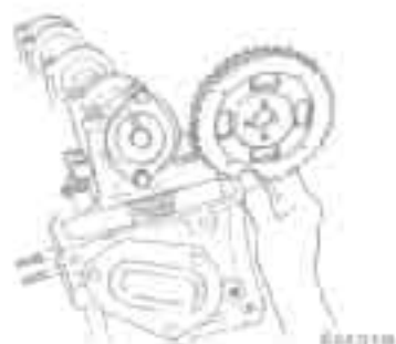
Fig. EM-80 Installing camshaft sprocket
