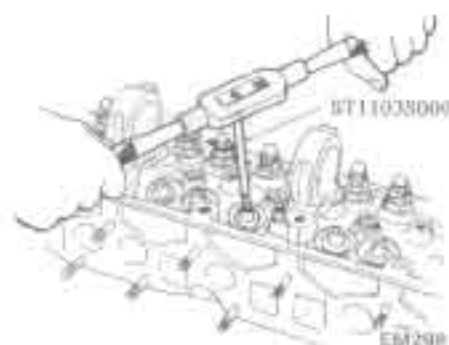
Fig. EM-3B Reaming valve guide
