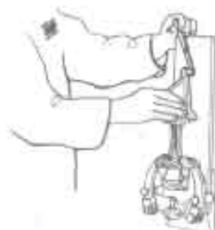
Fig. EM-56 Checking rod alignment
