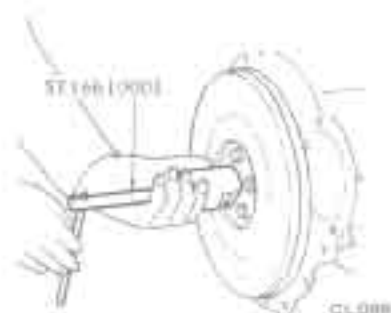
Fig. EM-61 Pulling out pilot bushing
