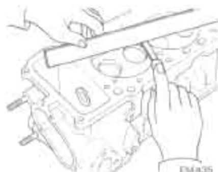
Fig. EM-30 Checking cylinder head surface
