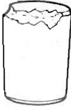
d) Cracked roller
