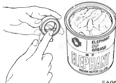
Fig. FA-23 Filling grease seal lip pocket with grease
