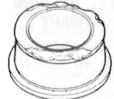
c) Cracked inner race
