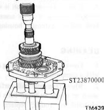
Fig. TM-31 Installing mainshaft assembly
