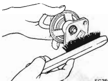
Fig. ET-42 Cleaning E.G.R. control valve
