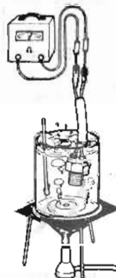
Fig. ET-36 Checking water temperature switch
