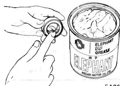
Fig. FA-21 Filling grease seal lip pocket with grease
