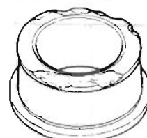
c) Cracked inner race
