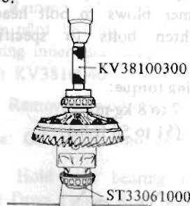
Fig. PD-20 Installing side bearing inner race
