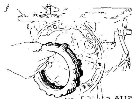
Fig. AT-63 Removing drive and driven plates
