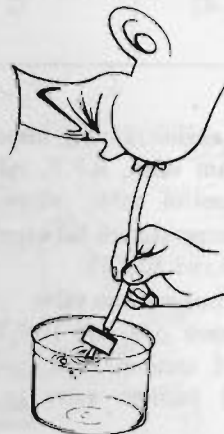
Fig. EC-28 Checking vacuum delay valve
