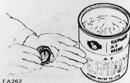
Fig. FA-18 Filling bearing cone with grease
