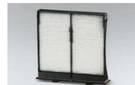
70 Air filter 72880FG000 Helps reduce dust and pollen infiltration into the vehicle cabin area. For the best result, it is recommended to replace the filter once a year or every 12,000 km. *For the replacement of originally equipped filter.
