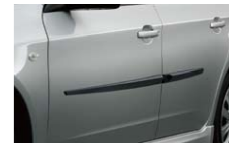
31 Side protector J105EFG100 Helps protect body side.
