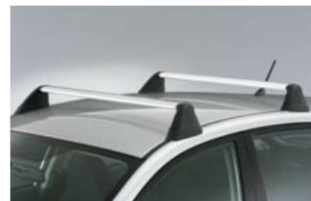
36 Aluminium carrier base E3610FG501 Perfectly fitting stylish base for carrier attachments.
