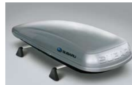
38 Transport box (Long) E361EYA900 Size: 2,267 x 805 x 355 mm. Volume: 430 litres. *Carrier base required.
