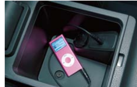
78 AUX outlet kit H6210FG000 A 3.5 mm auxiliary stereo mini-pin jack socket that allows you to listen to the sounds from portable music players. Now you can enjoy your own music through the car speakers. *For factory installed 1CD audio.
