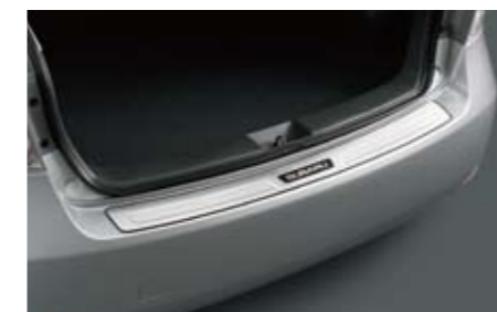
32 Cargo step panel (Stainless) E7710FG000 Protects rear bumper from scratches.
