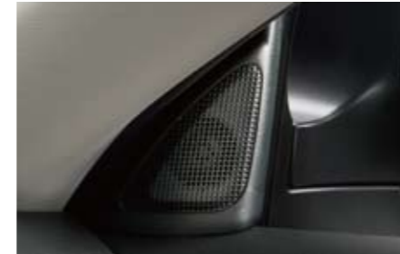
79 Tweeter kit H6310FG000 Special speakers enhance high-frequency audio. *For factory installed 1CD audio.
