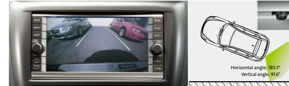
83 Rear view camera H0010FG000 High-resolution 250,000-pixel CCD camera that automatically displays the area around the rear of the car on the navigation screen when the reverse gear is selected. Has a horizontal angle view of 183.3° and a vertical angle view of 91.6°. *to be installed with NAVI.
