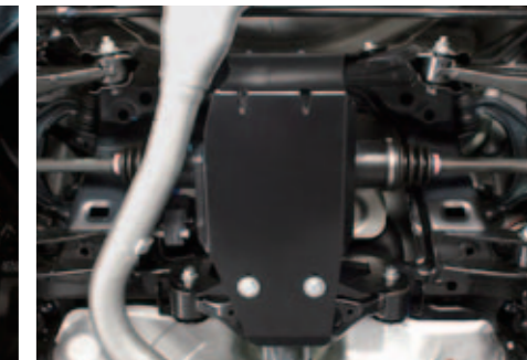
43 Rear Differential Under Guard E515EAJ300 Protect the underside of the rear differential.
