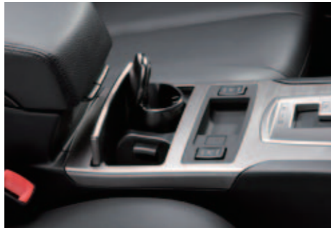
97 Ash Tray (in cup holder) 92172AG040 Interchangeable ashtray fits into the centre console cup holder.
