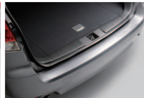
18 Rear Bumper Protection Foil E775EAJ100 Transparent film to protect the top of the bumper from scratches.
