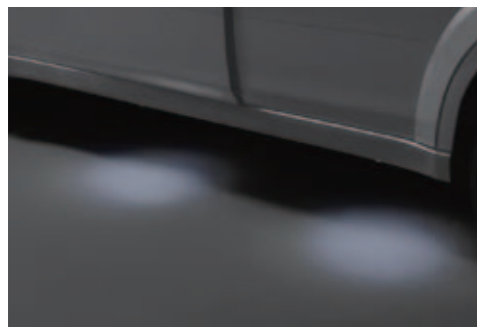
85 Puddle Lamps H471SAJ000 Located at the bottom of the vehicle and activates when door is opened.
