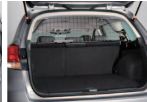
61 Dog Guard (K/M) F555EAJ000 Separates passenger's seats from the cargo compartment when carrying dogs.
