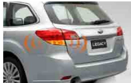
112 Tip blinking and safety hazard kit SEWAYA8000 Bi-functional safety item: side indicators blink 4 times and hazard lights are activated during emergency braking.
