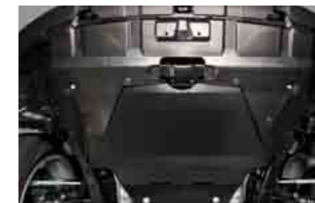
33 Engine Under Guard (Steel) E515EAJ000/E515EAJ020 Protects the engine sump from protruding rocks and stones.
