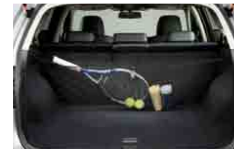
66 Net (Rear Seat Back) F5515AJ001 Can be stretched across the back of the rear seat to hold various types of cargo/luggage.
