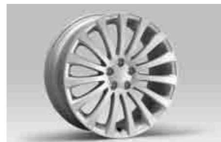
50 Alloy Wheel 15-spoke (18inch) 28111AJ040 18x7.5JJ offset 55
