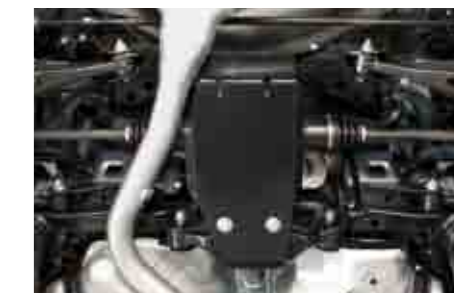
35 Rear Differential Under Guard E515EAJ300 Protects the rear differential from protruding rocks and stones.
