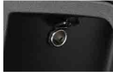
114 Cargo Socket H6710AJ100 Conveniently installed in the cargo compartment to supply 12VDC power.
