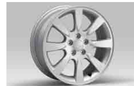
56 Alloy Wheel 8-spoke (16inch) 28111AJ100 16x6.5JJ offset 48
