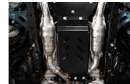
34 Transmission Under Guard E515EAJ200/E515EAJ220 Protects the transmission from protruding rocks and stones.
