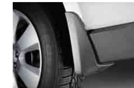
12 Splash Guard - rear set J1010AJ024 Prevents mud, snow, tar, rocks, etc. from being thrown up on the body.
