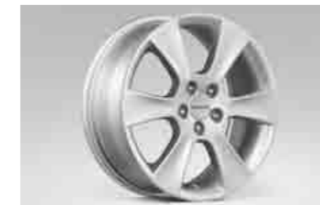
57 Alloy Wheel 6-spoke (16inch) SECWAG4001 16x6.5JJ offset 48
