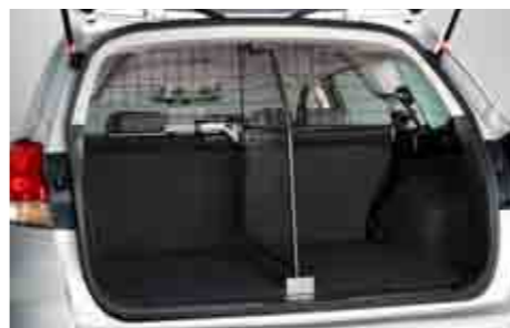
81 Dog Guard Divider (K/M) F555EAJ100 Separates the cargo room in 2 areas. To be used with dog guard (K/M).
