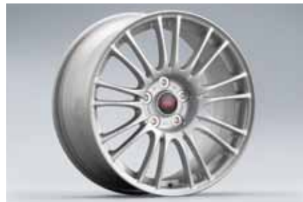
21 Alloy wheel 9-spoke, Silver (18 inch) 28111FG070 8.5"x18" offset 55 PCD 114.3 Tyre size 245/40R18
