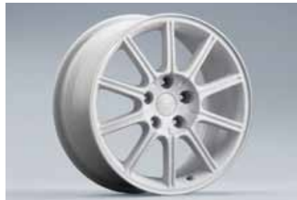
27 Alloy wheel 10-spoke, White (17 inch) 28111FE361 8"x17" offset 53 PCD 114.3 Tyre size 235/45R17
