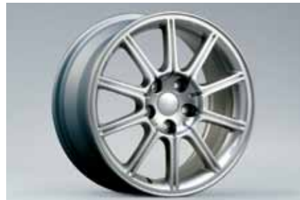
26 Alloy wheel 10-spoke, Silver (17 inch) 28111FE351 8"x17" offset 53 PCD 114.3 Tyre size 235/45R17
