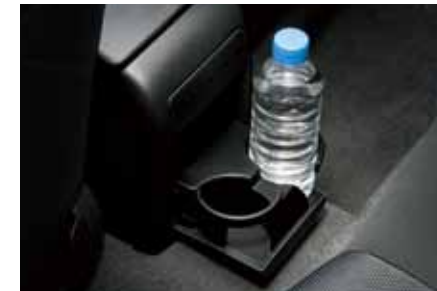
57 Rear cup holder (Black) J2010FG010JC Cup holder for the rear passengers that can be neatly stored at the back of the centre console.
