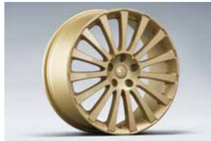
19 Alloy wheel 15-spoke, Gold (19 inch) SECWFG4020 8.5"x19" offset 55 PCD 114.3 Tyre size 245/35R19
