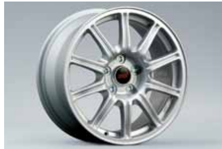
24 Alloy wheel 10-spoke, Silver (17 inch) 28111FE272 8"x17" offset 53 PCD 114.3 Tyre size 235/45R17
