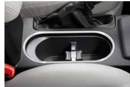
45 Chrome Cup Holder Surround J205ESG000 Chrome frame that gives a highlight to the center console.
