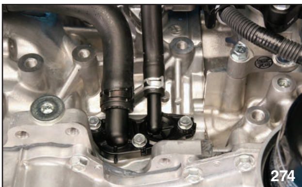
COOLANT AND PCV HOSES MOUNTED
