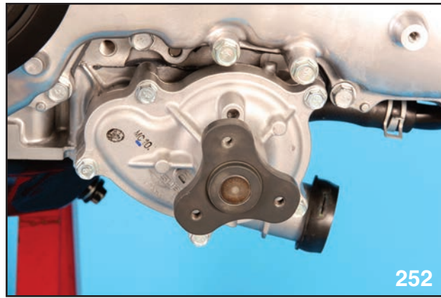
WATER PUMP FRONT VIEW
