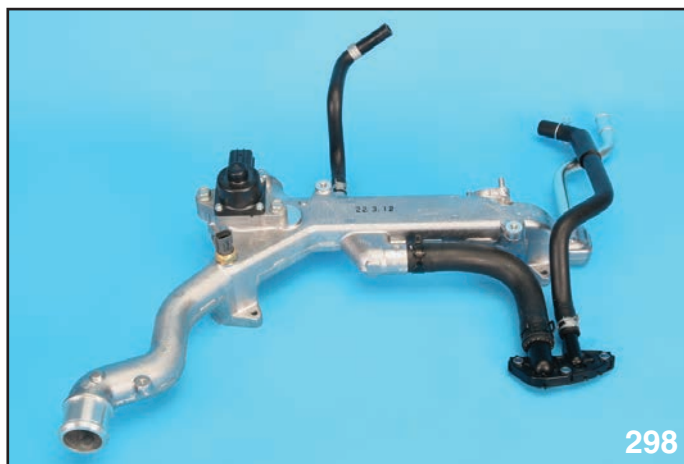
COOLANT CROSSOVER PIPE FRONT VIEW
