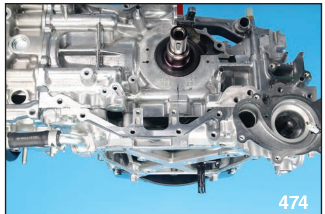
OIL STRAINER — REMOVED
