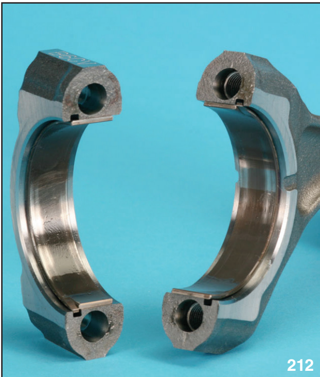
CONNECTING ROD CAP SEPARATED FROM ROD
