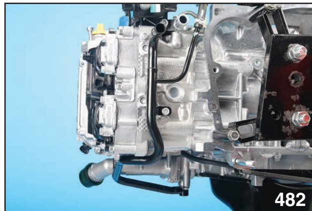
LOWER WATER PIPE (REAR VIEW)
