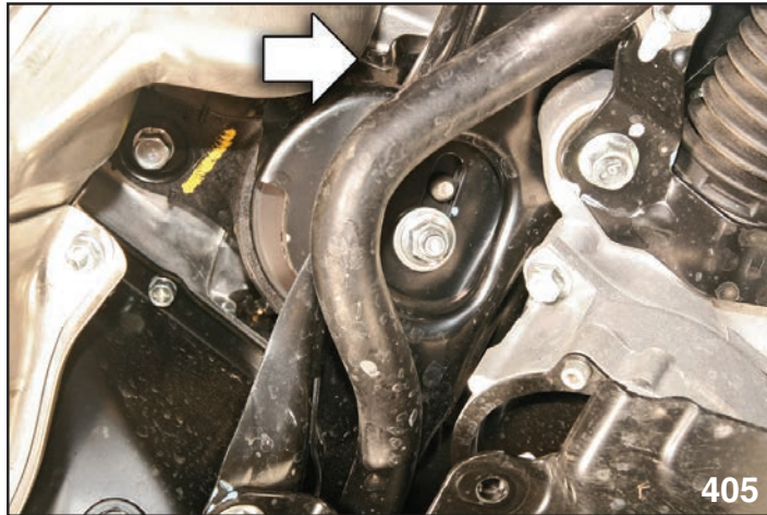
OIL LEVEL SENSOR
