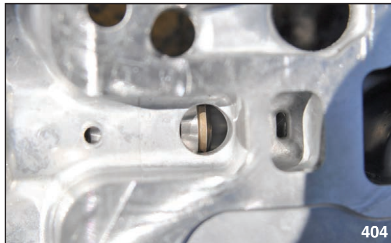
RELIEF VALVE AT 2 ND OPENING
