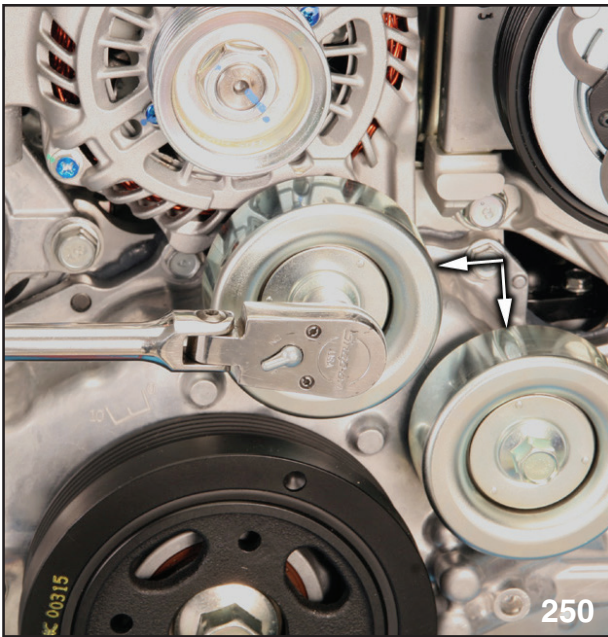
REMOVING BELT IDLER
