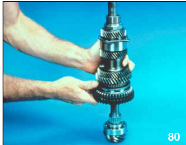
INSTALL DRIVEN SHAFT ASSEMBLY
