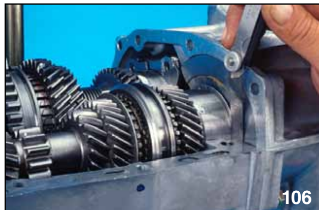
MAIN SHAFT END PLAY CLEARANCE
