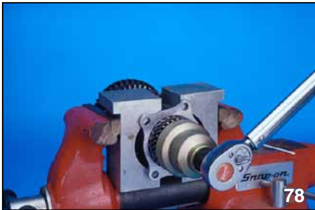
INSTALL DRIVEN SHAFT WASHER AND LOCK NUT
