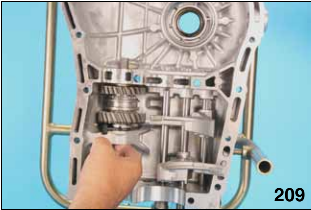
INSTALLING THE REVERSE IDLER GEAR ASSEMBLY
