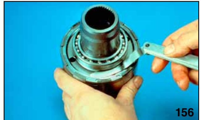
MEASURING SNAP RING CLEARANCE
