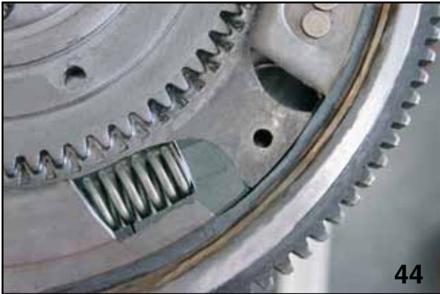
ACTUATOR IN CONTACT WITH SPRING CARRIER
