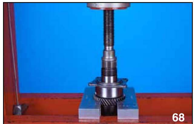
PRESS ROLLER BEARING AND 3RD-4TH GEAR ASSEMBLY
