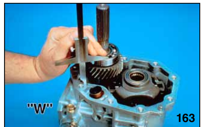
MEASURING HEIGHT "W"
