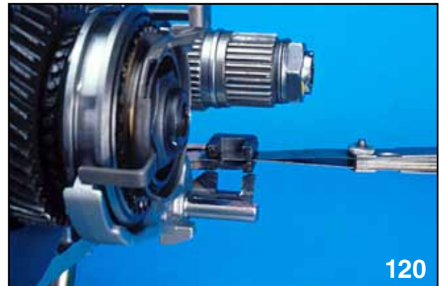
MEASURE SHIFT ROD END CLEARANCE
