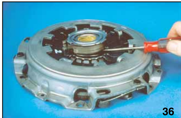
RELEASE BEARING REMOVAL
