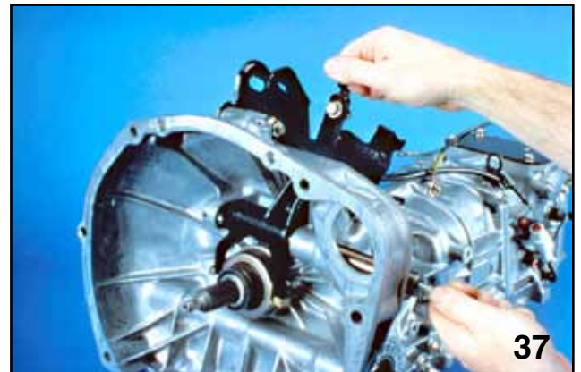
RELEASE BEARING INSTALLATION
