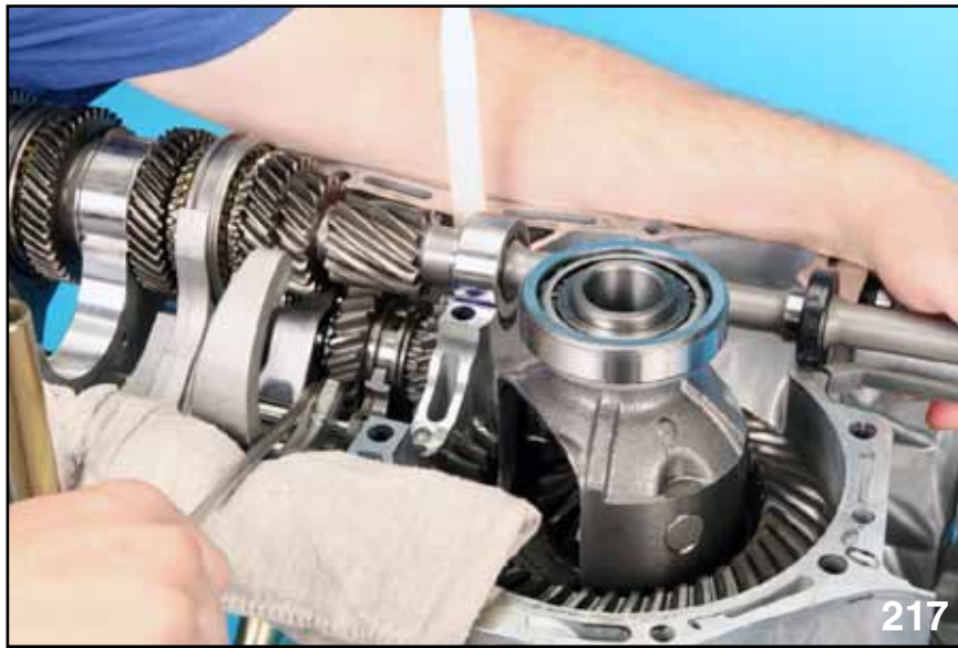
PRE-LOADING THE SUB-GEAR
