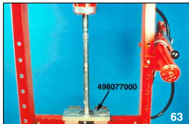
PRESS PINION SHAFT BEARING AND WASHER
