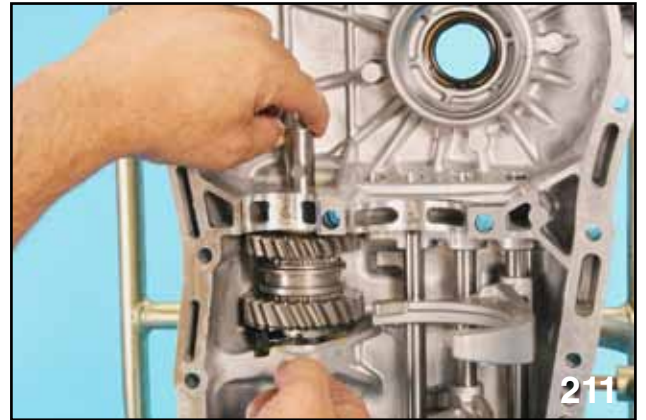
INSTALLING THE REVERSE IDLER SHAFT BUSHING
