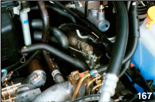
PHV (PRESSURE HOLD VALVE)
