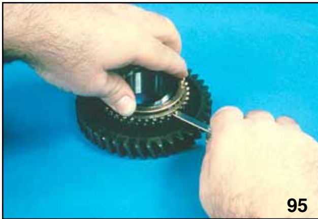
SYNCHRONIZER RING WEAR
