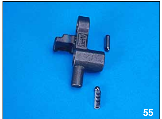
REVERSE FORK ROD ARM, PIN, BALL AND SPRING
