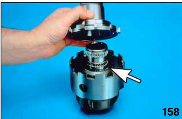
REASSEMBLE CENTER DIFFERENTIAL ADJUSTING WASHER
