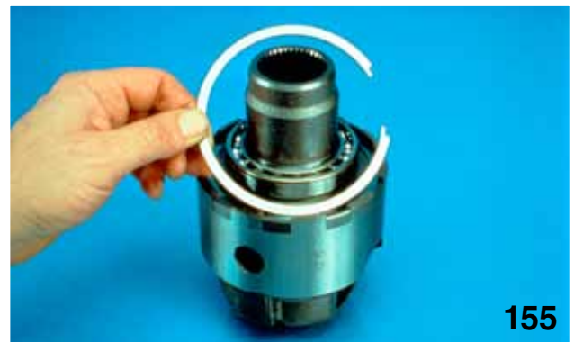
CENTER DIFFERENTIAL HOUSING SNAP RING CLEARANCE
