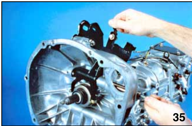
RELEASE FORK SHAFT REMOVAL
