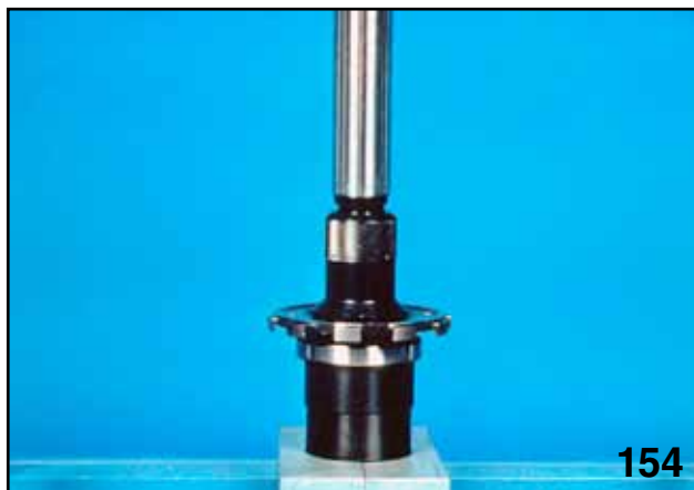
INSTALL CENTER DIFFERENTIAL BALL BEARING
