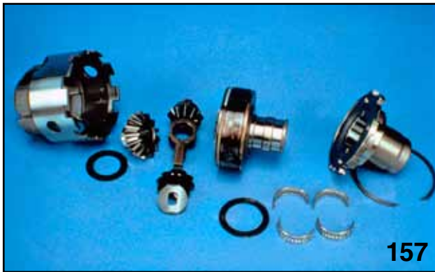
REASSEMBLE CENTER DIFFERENTIAL
