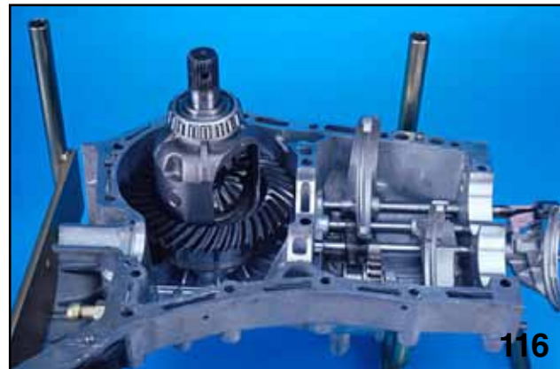
INSTALL DIFFERENTIAL ASSEMBLY
