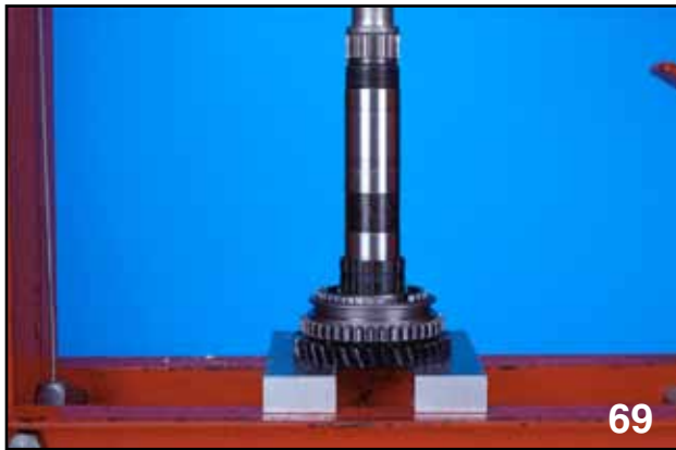
PRESS 1ST AND REV GEAR ASSEMBLY
