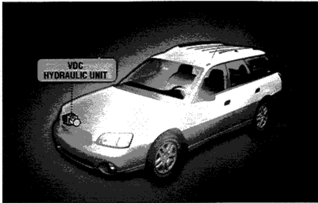
Location of VDC Hydraulic Unit
