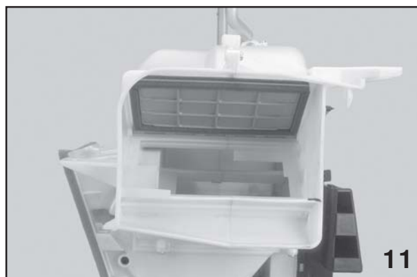
Heater Door closed
