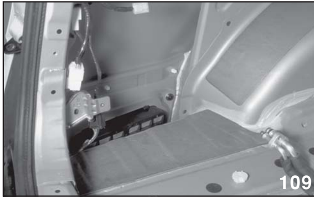
Rear Evaporator Removed
