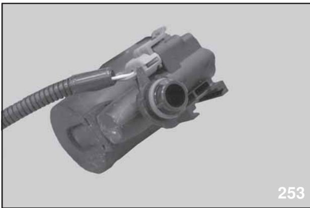
Drain Valve Separated from Canister (NOT SERVICEABLE)
