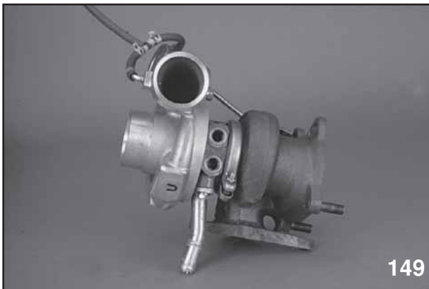
Coolant Connection and Oil Return
