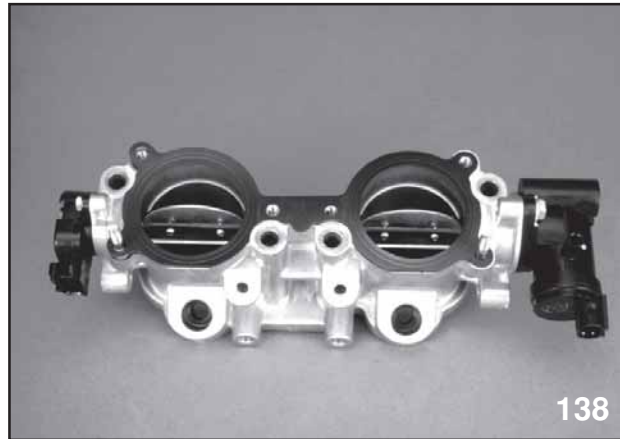
Tumble Generator Valve Rail
