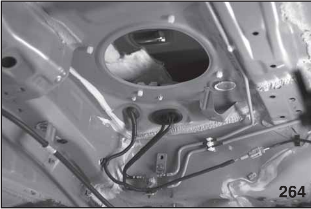
Tank Removed, Main Pump Access
