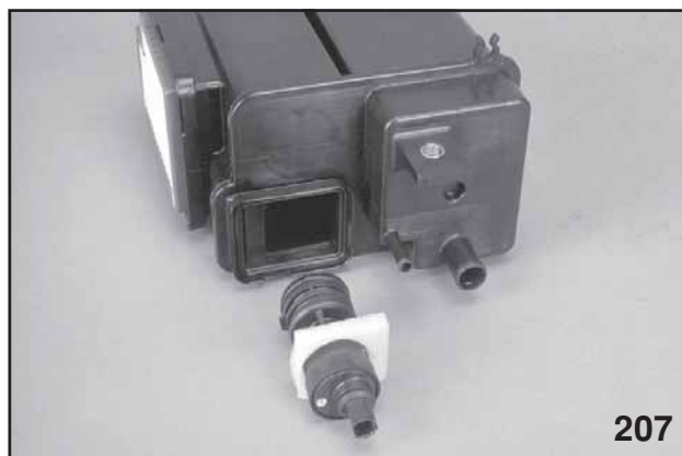
Drain Valve Separated from Canister (NOT SERVICEABLE)
