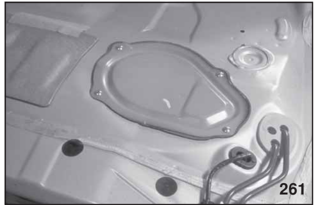
Sub Pump Access
