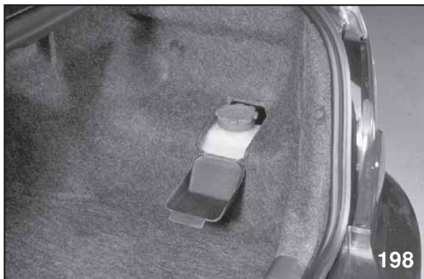
Normal Access to the Water Tank
