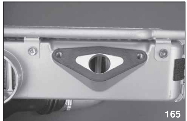
Bypass Valve Connection
