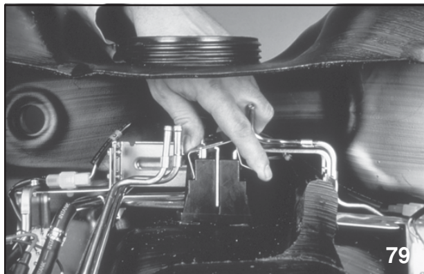
Removing Fuel Pump
