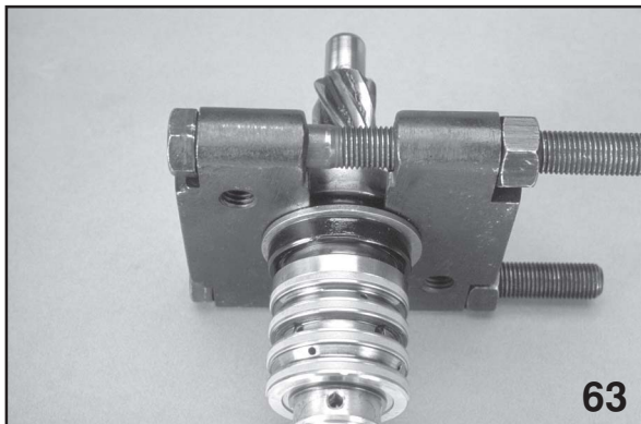
Removing Lower Bearing
