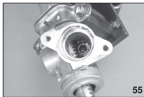
Control Valve Removed
