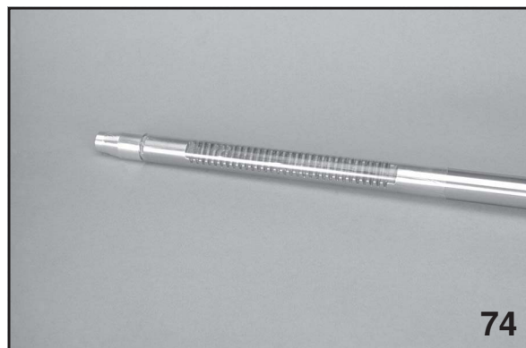
Rack Cover installed
