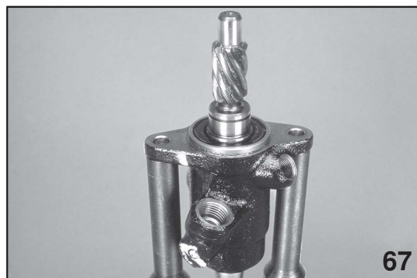
Installing Rotary Control Valve
